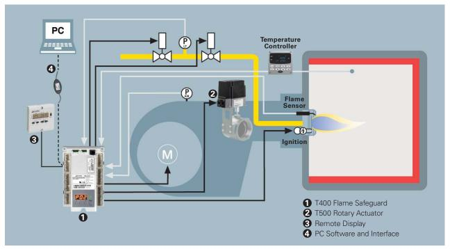
Typical modulating gas burner control system with a T400 Flame Safeguard
